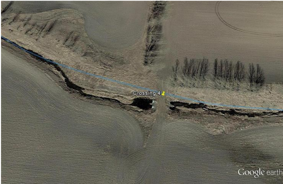
Figure 20: Crossing 4: potential fish barrier, especially under low flow conditions, due to improperly sized or sloped culvert. Imagery taken on 4/14/2015.
