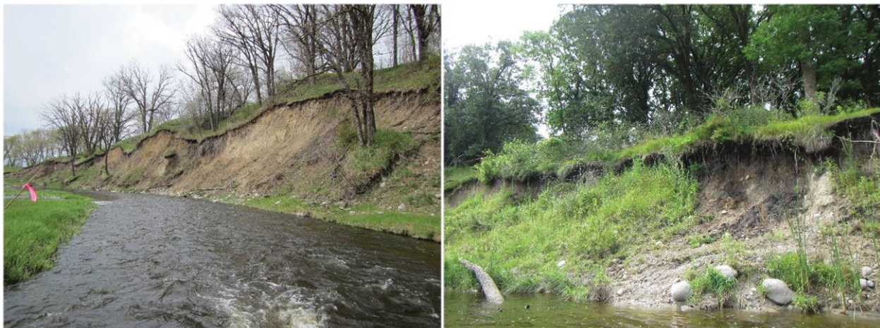
Figure 33. Images of bank erosion at Station 94RD012 along AUID 650 on May 19, 2014 (left) and July 24, 2014 (right).
