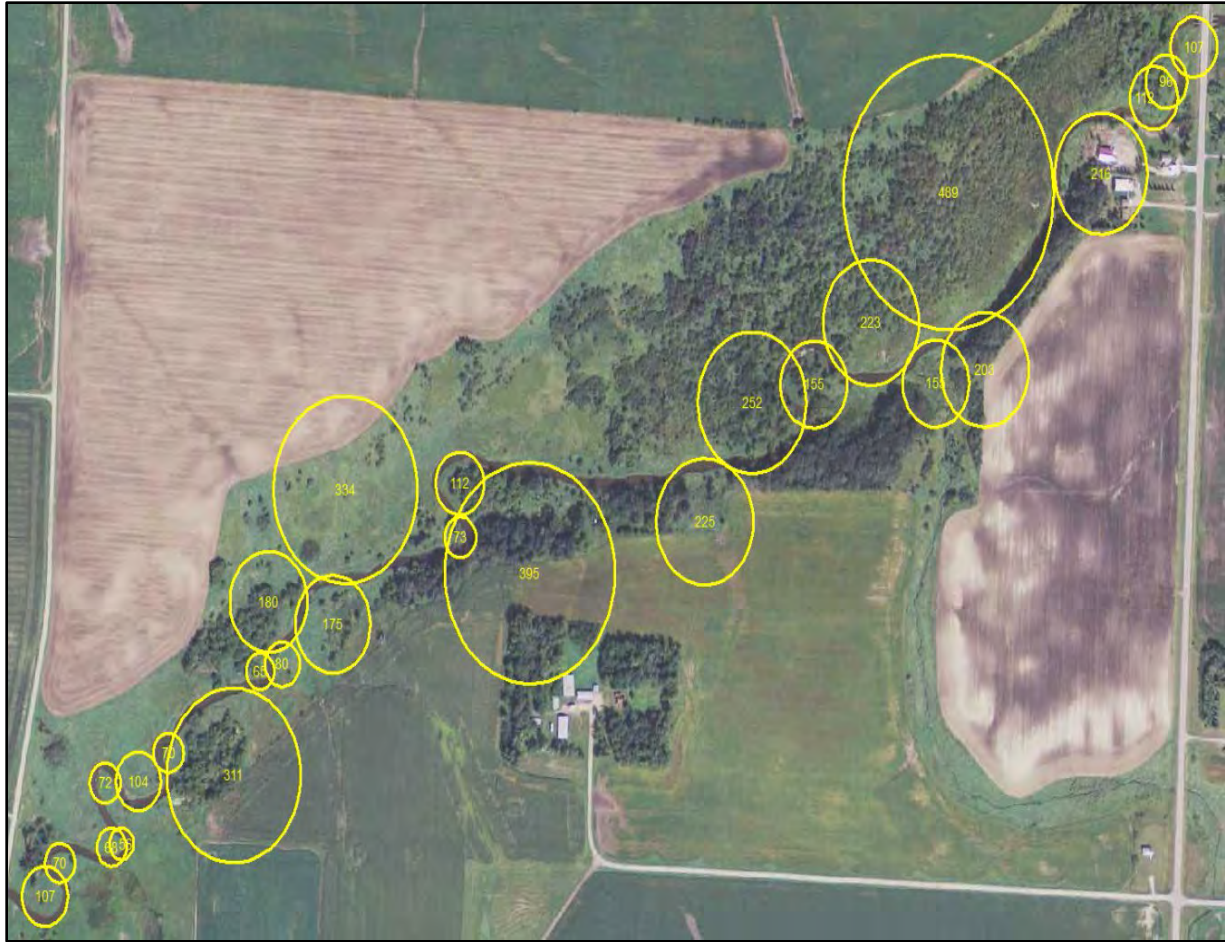
Figure 23. Near bank stress estimates using radius of curvature (yellow labels are radii of red or yellow circles that fit stream bends) divided by Wb_{kf} .
