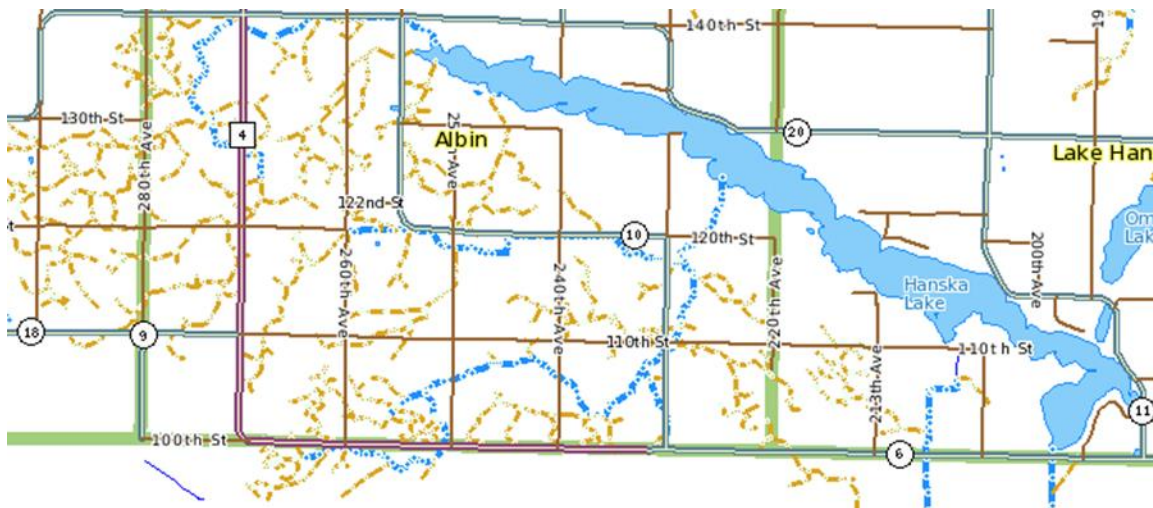
Figure 295. Lake Hanska - Network of Ditches (blue) and Drain tile (brown) from Brown County GIS website, 2015.
