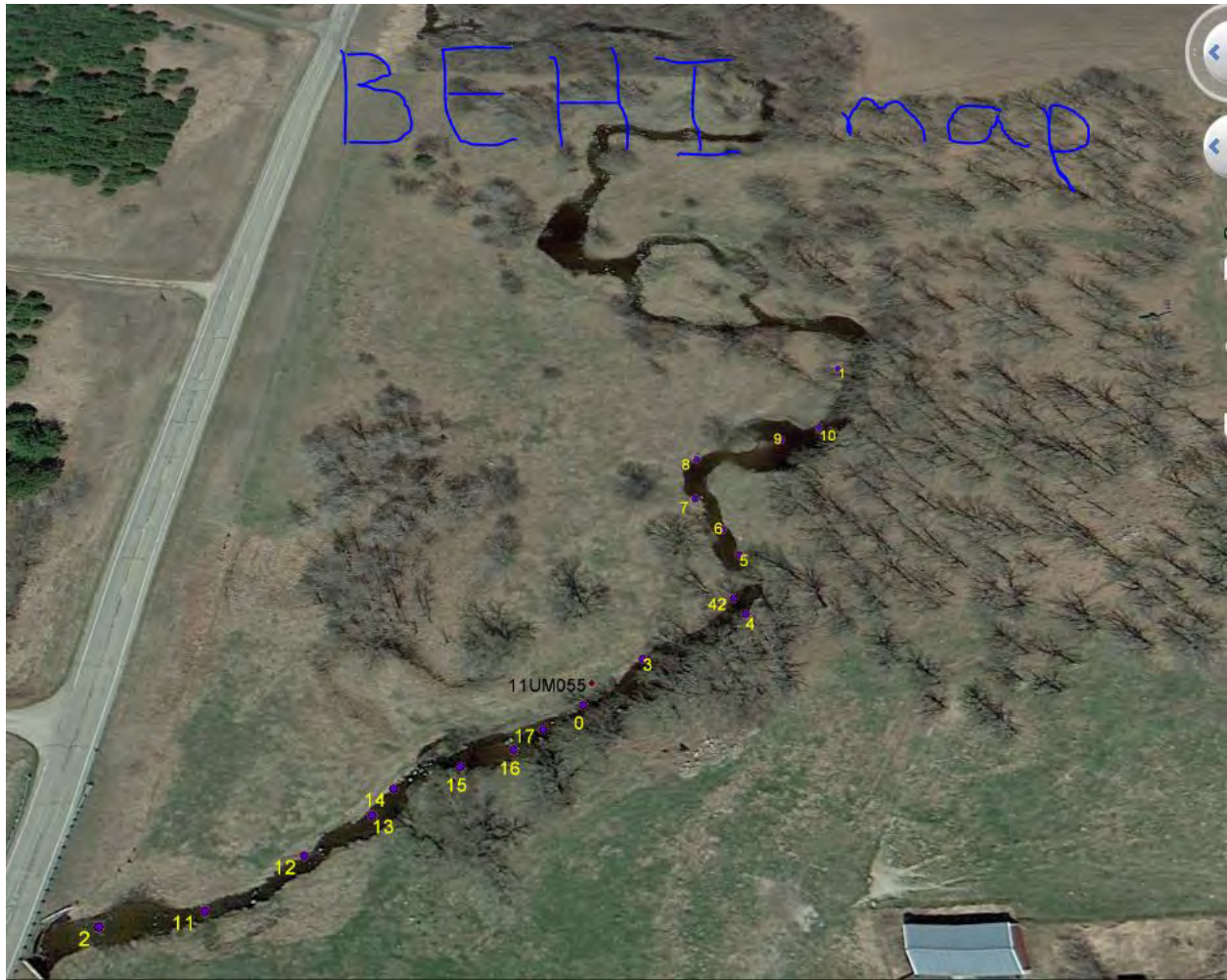
Figure 7.0.4: Biological site 11UM055 location map of bank erosion areas used in calculation of BEHI.
