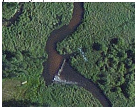
Photo 15: Possible barrier with turbulent overflow
