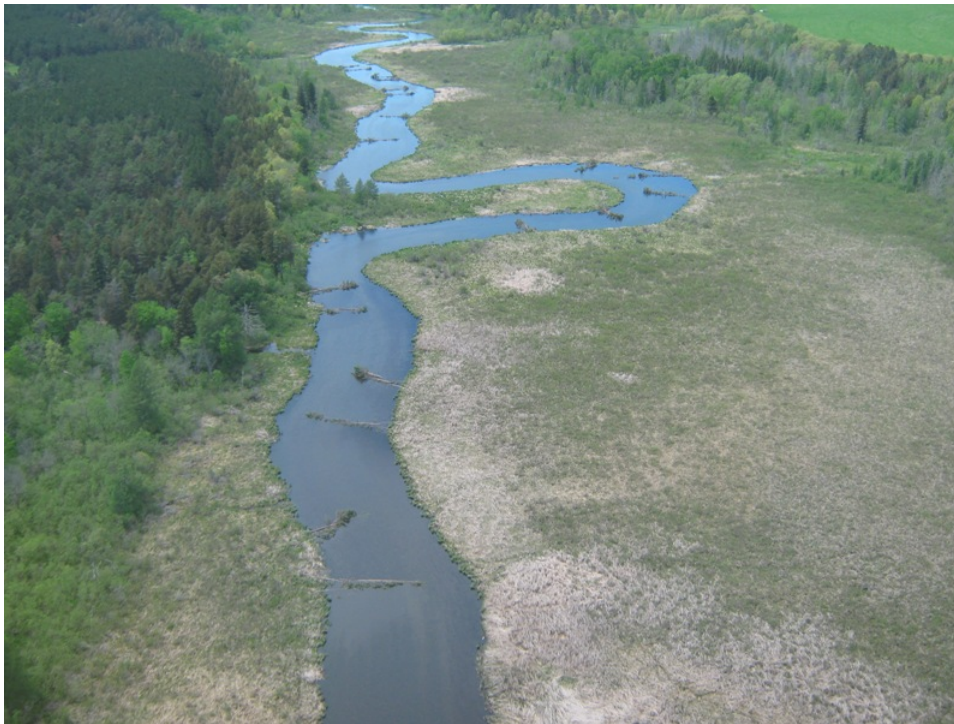
Photo 14. Placement of imported trees intended to deepen the thalweg, narrow the channel, add sinuosity, and add cover for fish. Again note the natural wide sedge meadows that occur in this region. MDNR Photo
