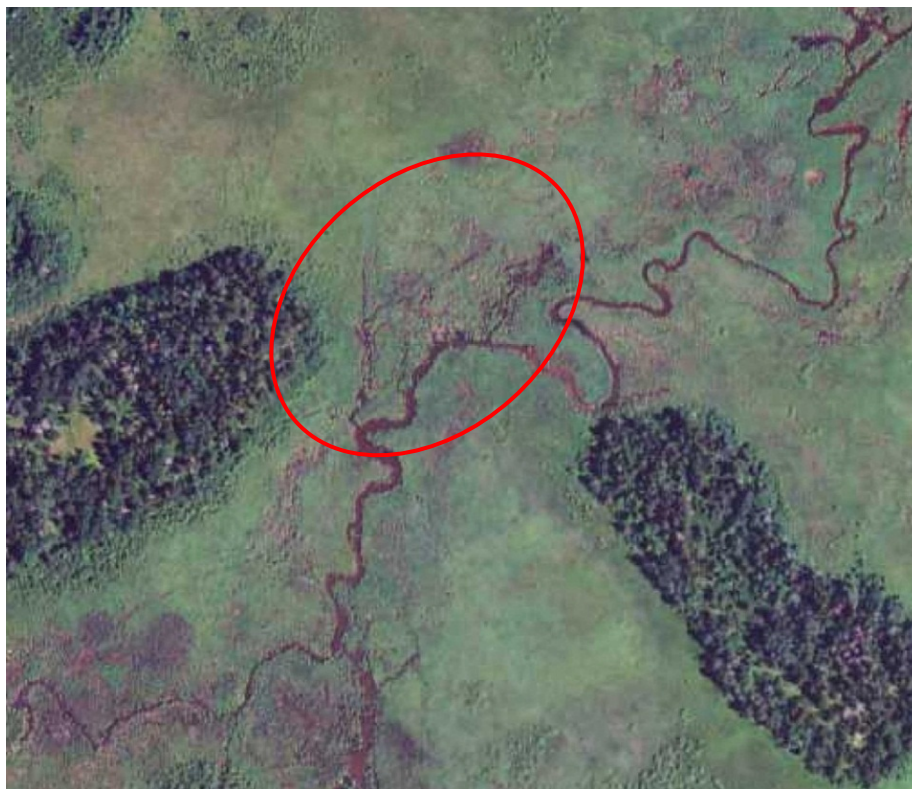
Photo 3. Farnham Creek groundwater seeps. The circled area shows shallow groundwater seeps emerging within the sedge meadow and entering Farnham Creek. Also note the orange color seen in many places along the channel due to iron inputs from groundwater.
