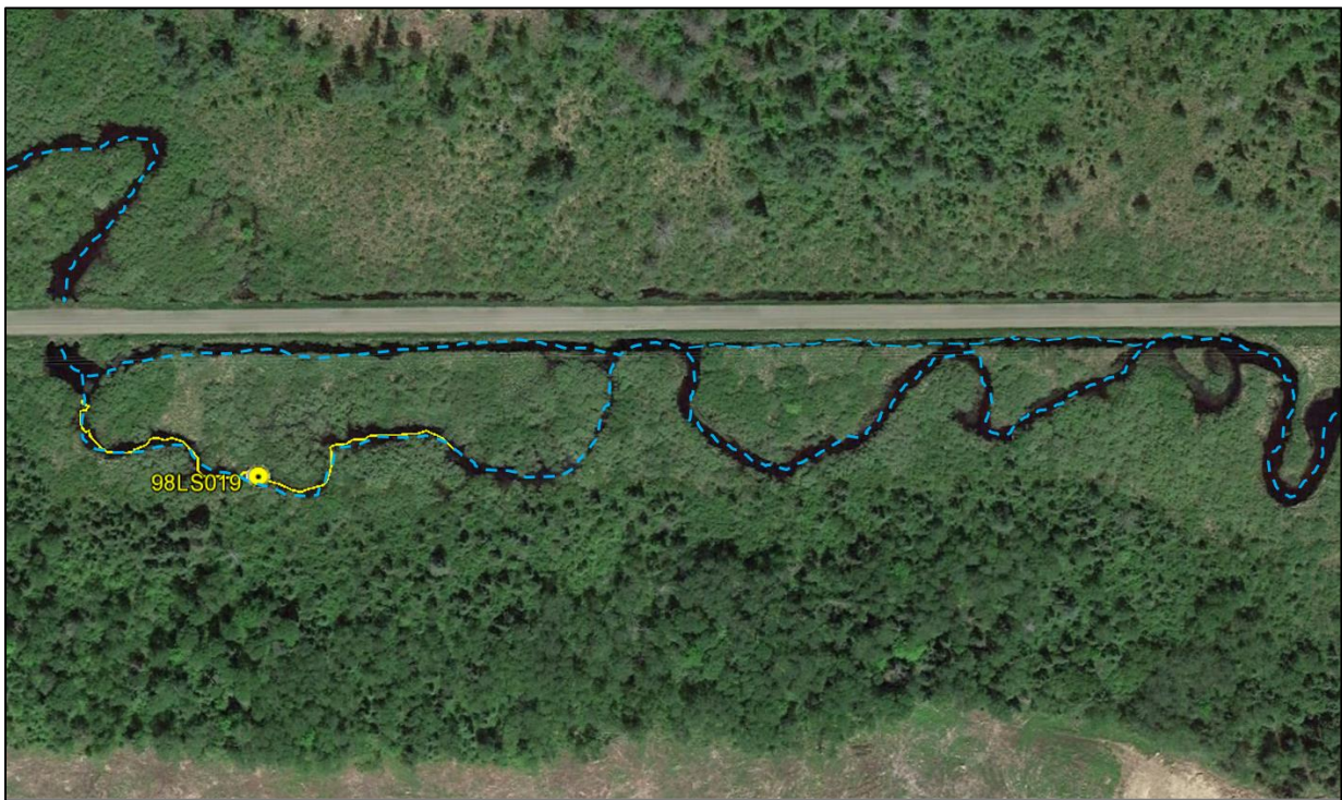
Figure 27. Aerial photo of station HC 3.2 (98LS019) of Hellwig Creek showing the road ditch adjacent to the natural channel. This ditch diverts flow during all flow conditions. Yellow line indicates the reach that was sampled by biological monitoring crews.
