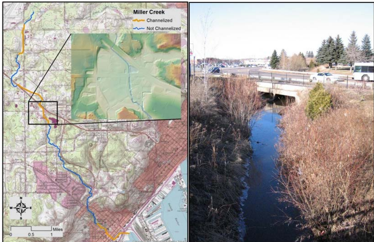
Figure 71: Map showing the channelized and straightened reaches of Miller Creek
