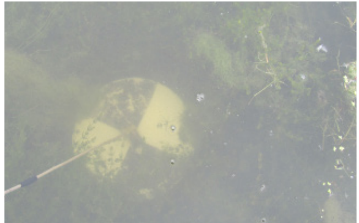
One way to measure clarity of water is to use a Secchi disk on a rope marked with centimeters, dropping the disk into the water until it can no longer be seen. Secchi readings in Bear and State Line lakes show low water clarity due to excessive algae and plant growth.
