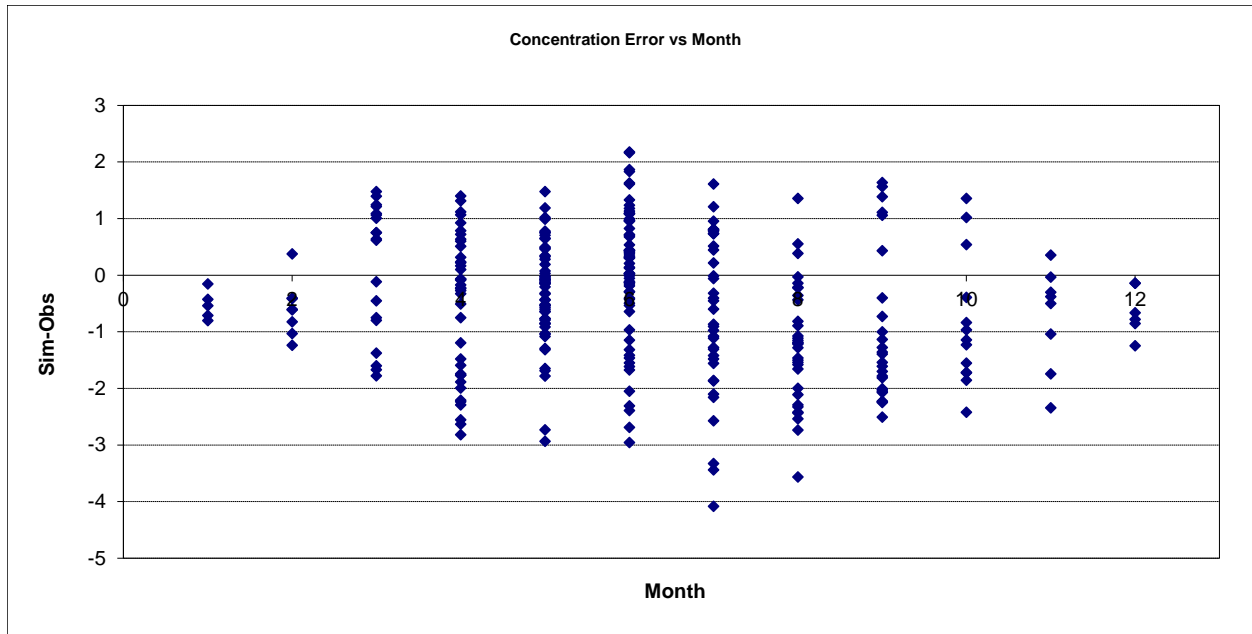
Figure 454. Residual (Simulated - Observed) vs. Month Total Kjeldahl Nitrogen (TKN) at West Fork Des Moines River at Jackson
