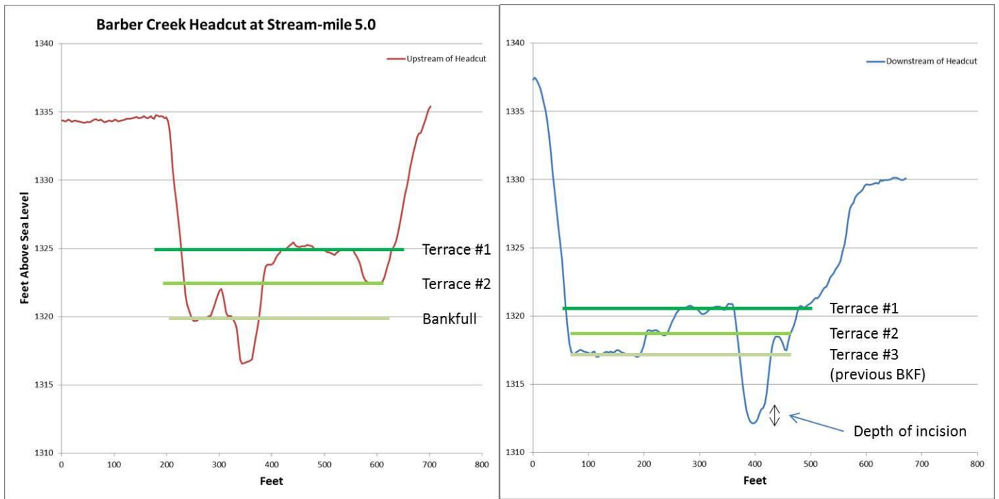
Figure 37: Cross-sections of Barber Creek, located above and below a suspected headcut.
