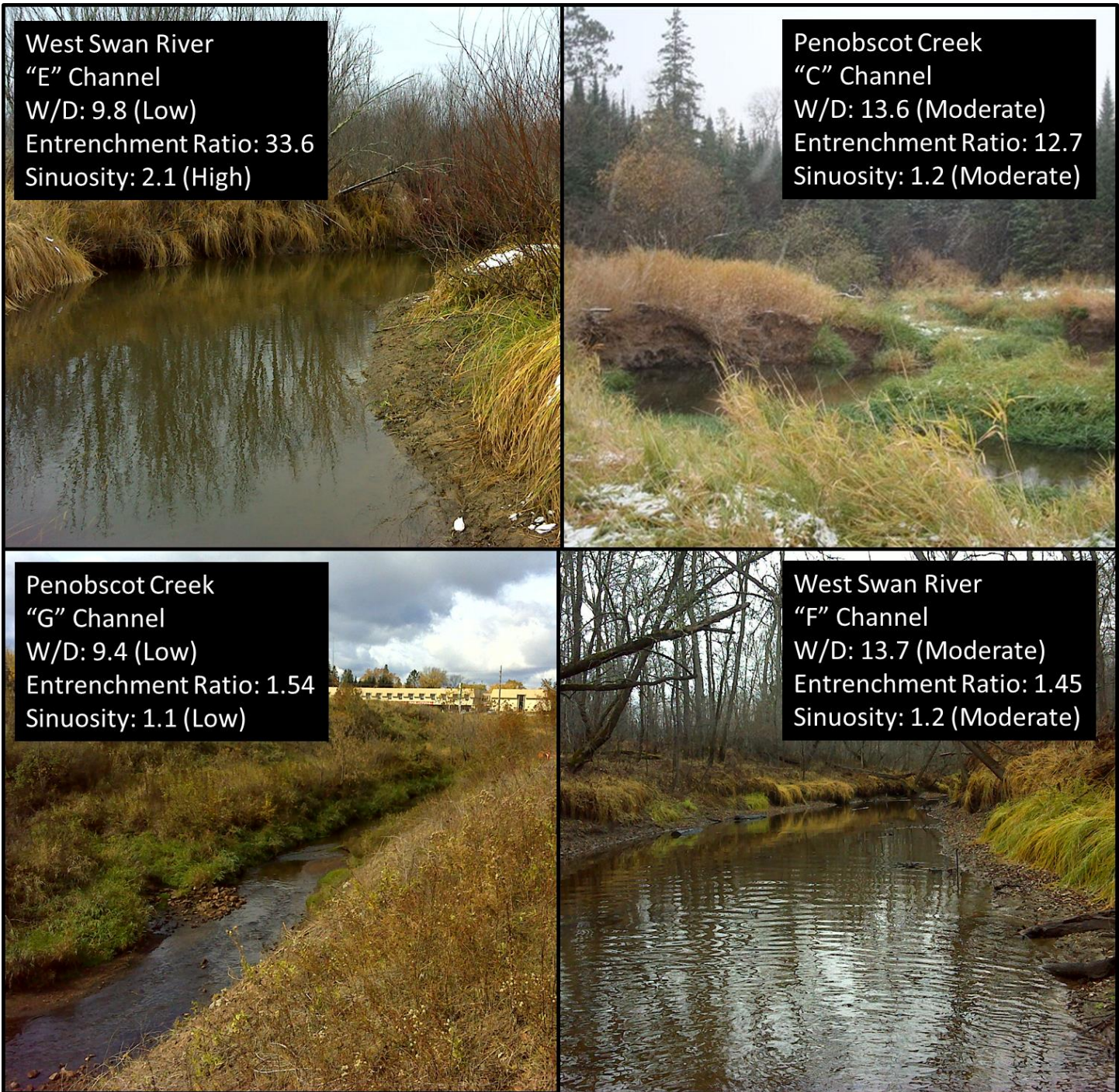
Figure 20: Examples of each of the four stream types documented in the Swan River watershed
