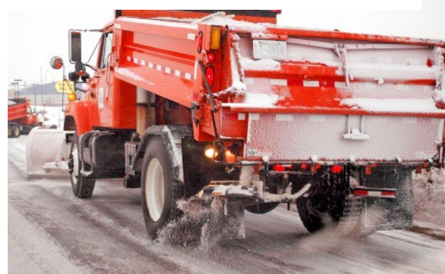
Figure 10. Road salt application
