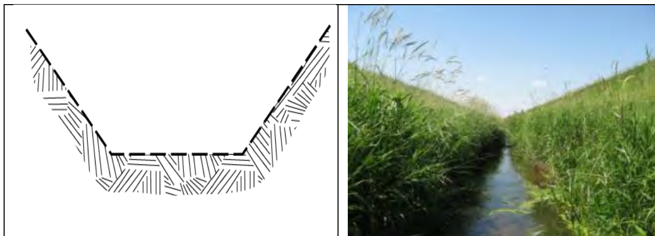
Figure 7: Cross-section of trapezoidal ditch design (left) and an example of this ditch design in Sauk River watershed (right).
