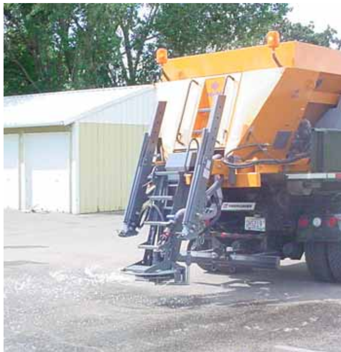
Figure 5 – Mn/DOT truck equipped with epoke, state of the art equipment for prewetting and anti-icing applications.
