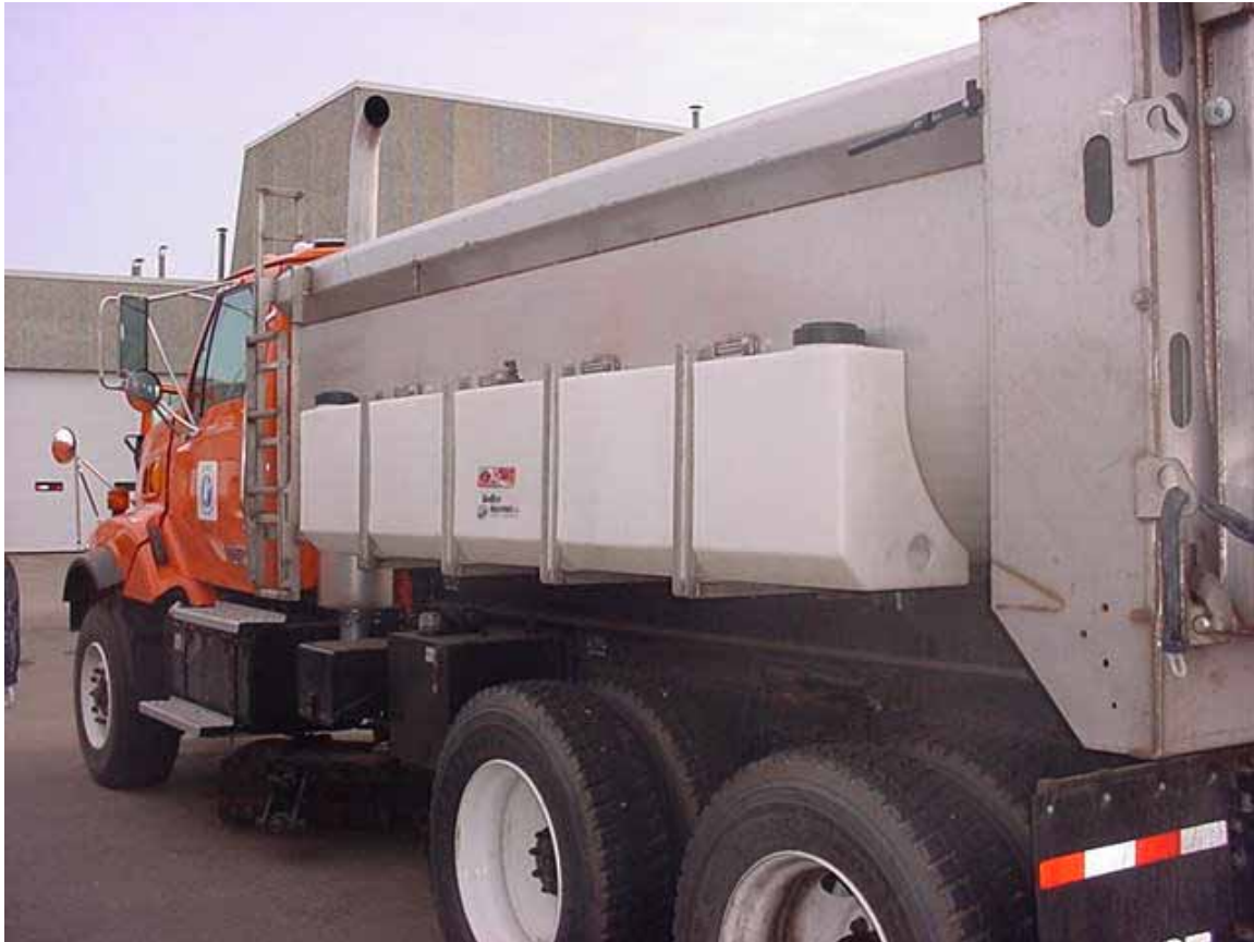
Figure 6 – Mn/DOT truck equipped with pre-wetting equipment.
