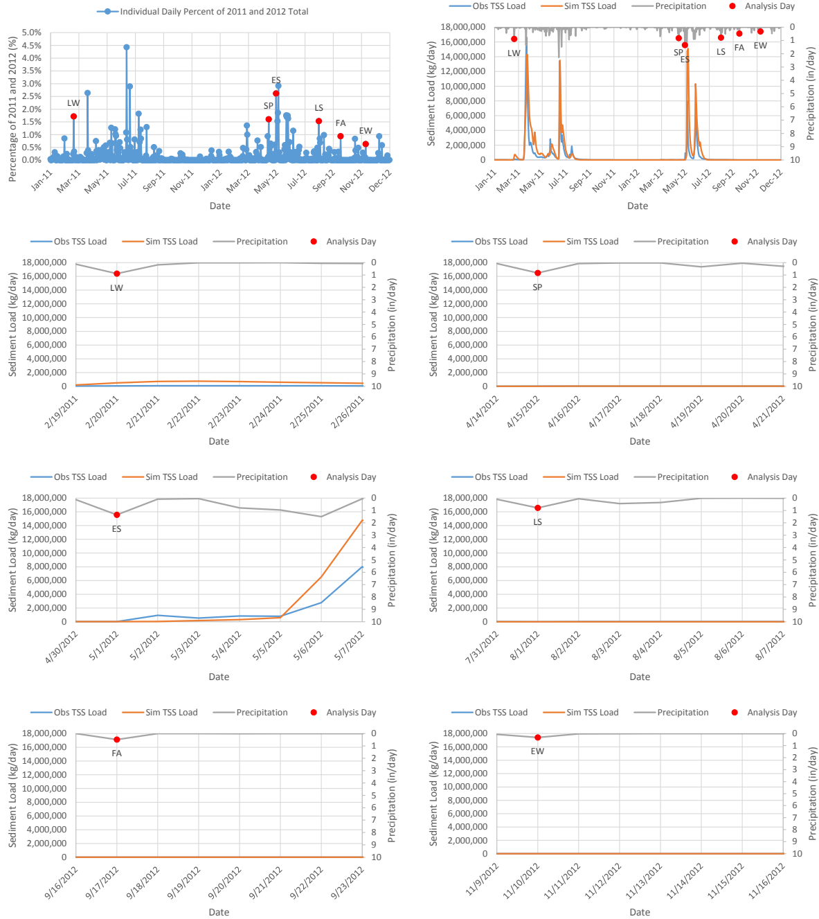
Figure 33. Time Series Plots for Largest Hourly Precipitation Days for Cottonwood River near New Ulm, MN68
