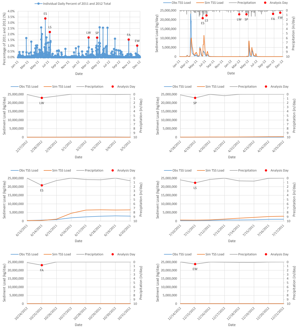
Figure 41. Time Series Plots for Largest Daily Precipitation Days for Blue Earth River near Rapidan, MN
