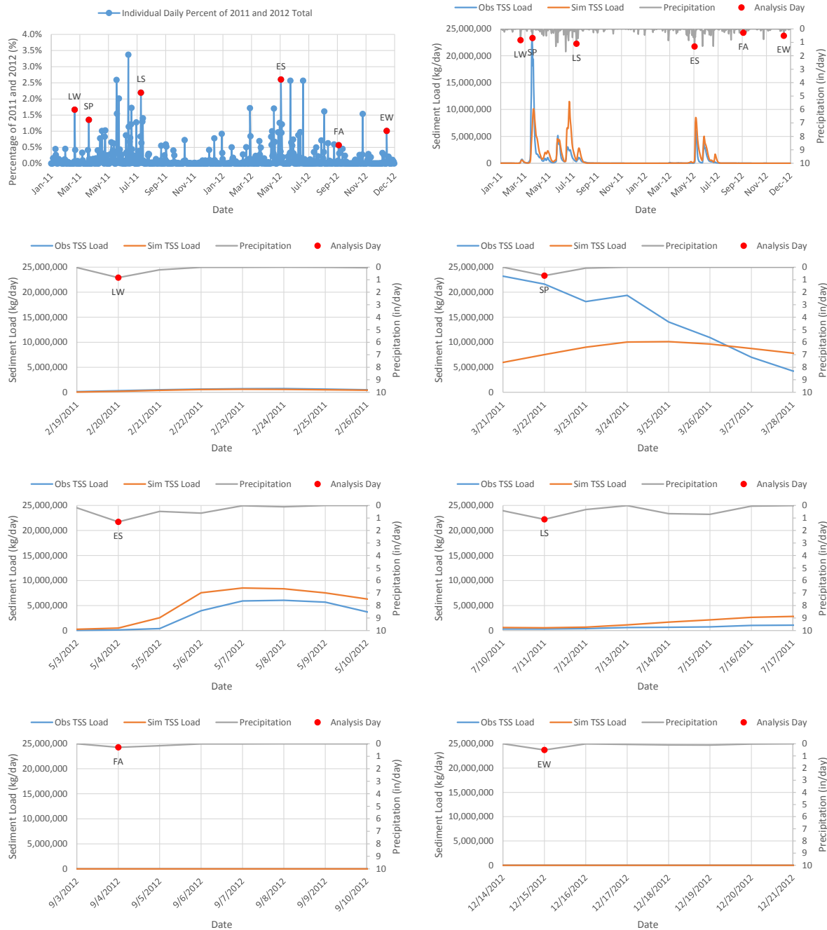
Figure 42. Time Series Plots for Largest Hourly Precipitation Days for Blue Earth River near Rapidan, MN
