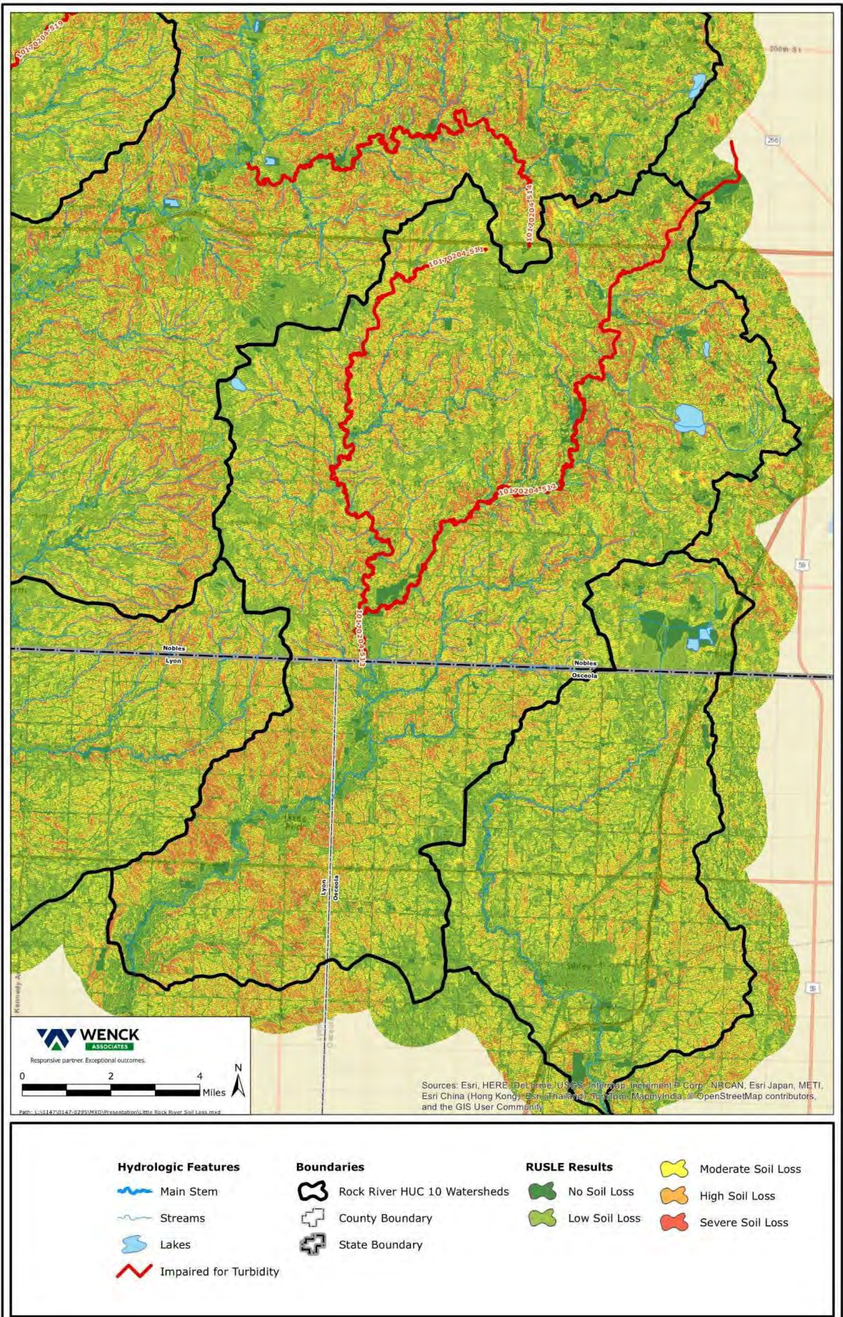
Figure B-15. Little Rock River Subwatershed (Rock River Watershed) potential soil loss (RUSLE).
