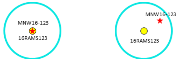
Figure 2. Example MWCA GPS points. POINT = red star, CENTER = yellow circle, Site boundary = light blue. Note the different naming conventions of the POINT and CENTER. For the Standard Circular Site (upper-left), the POINT and CENTER coordinates are equal. The Standard Circular Site-Shifted (upper-right) clearly illustrates the difference between the POINT and the CENTER.
