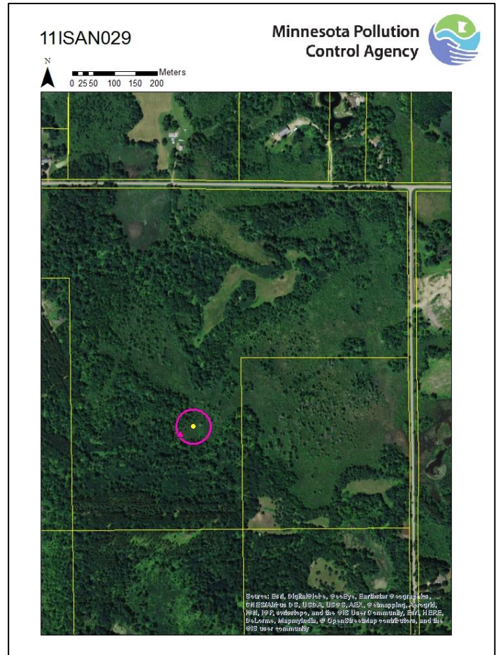
Figure 3. Example access map for a MWCA Site. The view includes roads and is centered on possible foot routes to the Site. Coverages include: Sample Site boundary (pink), POINT (pink triangle), CENTER (yellow point), ownership parcels (yellow line-work, landowner labels were de-activated for example). Appropriate labels included in the header.
