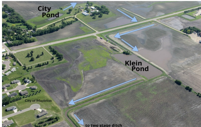
A drainage improvement project on Blue Earth County Ditch No. 57 (CD 57) helps control flows and improve water quality of drainage water from agriculture and stormwater from the City of Mapleton. Photo: ISG Architecture, Engineering, Environmental, and Planning.
