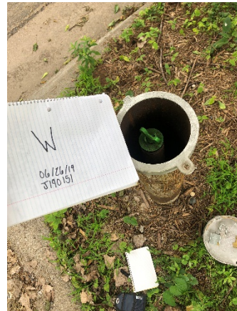
Photo 2 Well W located at 22 nd and Talmadge. PVC well casing and plug present. No bollards.
