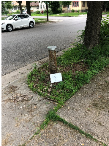
Photo 33- Well W. 2" PVC well casing, plug present, three bollards. *Two W well IDs this one located on 8th St.
