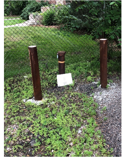
Photo 14- Well B. - ~2" PVC well casing, plug/cap present, two bollards and surrounded by fence to the south
