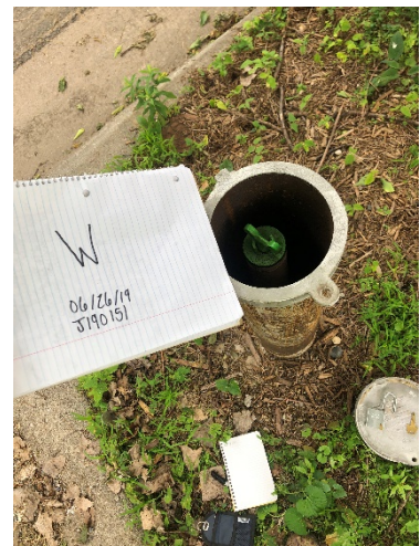
Photo 34- Well W. 2" PVC well casing, plug present, three bollards. *Two W well IDs this one located on 8th St.
