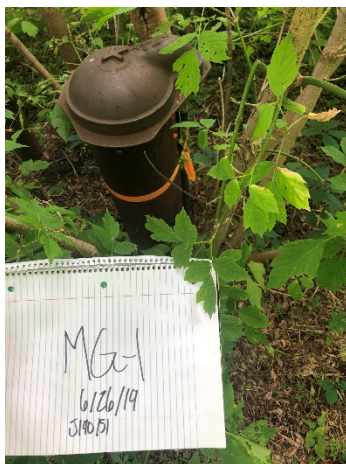
Photo 17 Well MG-1. Hidden under vegetation and behind a tree. Two bollards present, one appears to have been backed into and is slightly bent.
